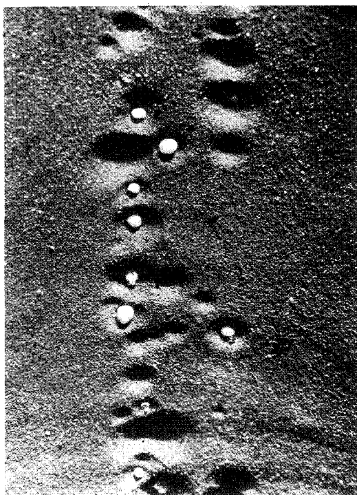
Fig. 10 Web part of the extinguished combustion surface of 200° spinning motor. 5
